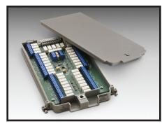
The Model 7702 plug-in module offers 40 channels of 2-pole or 20 channels of 4-pole multiplexer switching that can be configured as two independent banks of multiplexers. The Model 7702 provides two additional protected channels for current measurements. It is ideal for RTD, thermistor, and thermocouple temperature applications.
